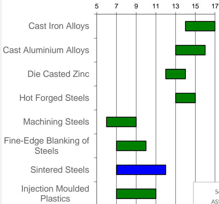
Typical tolerance rangers (IT) for various materials and manufactorig processes
