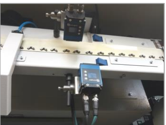
CAMERA CONTROL DIRECTLY IN THE PRODUCTION
